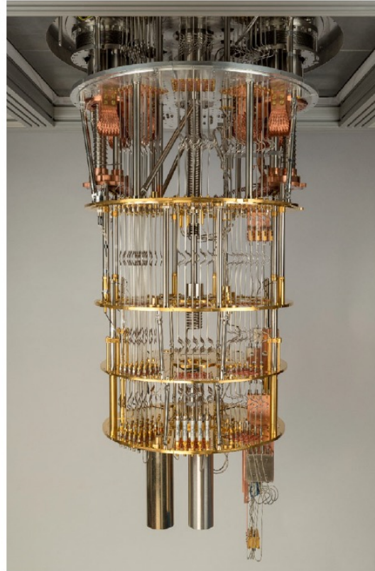
Figure 3 Cabled dilution refrigerator (DR). (a) Bluefors XLD DR with 25 drive lines, 25 flux lines, 4 read-out, 6 read-in, and 5 pump lines installed (see end of Sect. 3.1 for details). (b) Schematic of the cabling configuration within the DR
